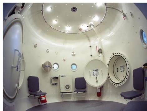
Figure: 16 A multiplace chamber to treat multiple individuals with hyperbaric oxygen.
