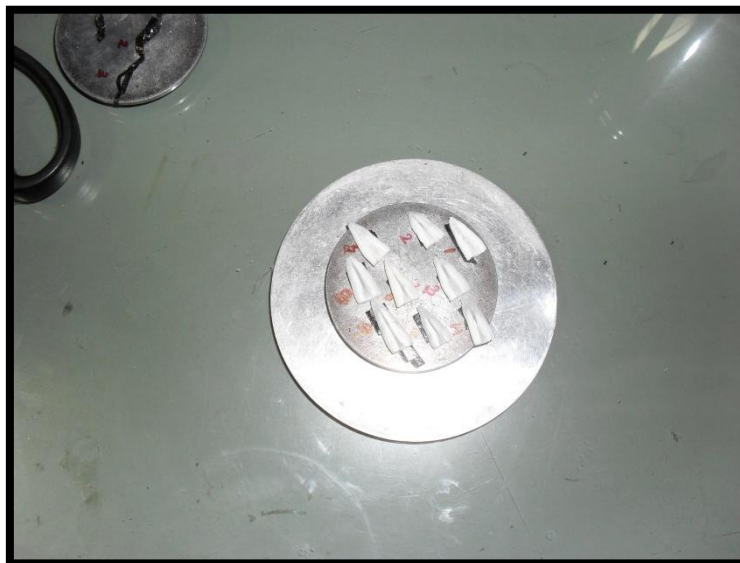
Fig.16: GOLD SPUTTERED TEETH SAMPLES
