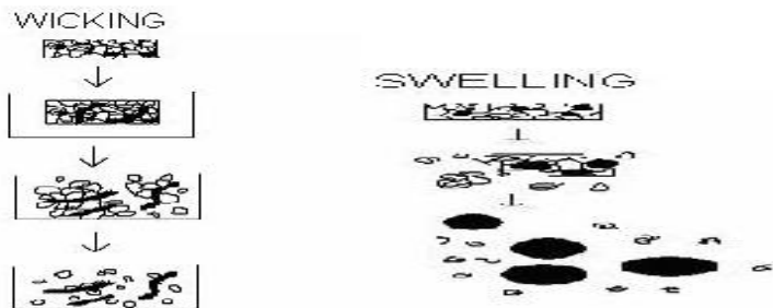
Figure: 1.8. Mechanism of capsule disintegration by wicking and swelling
