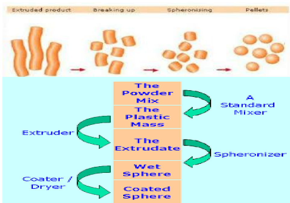
Fig1.11 Steps of pellet formation by Extrusion-spheronization
