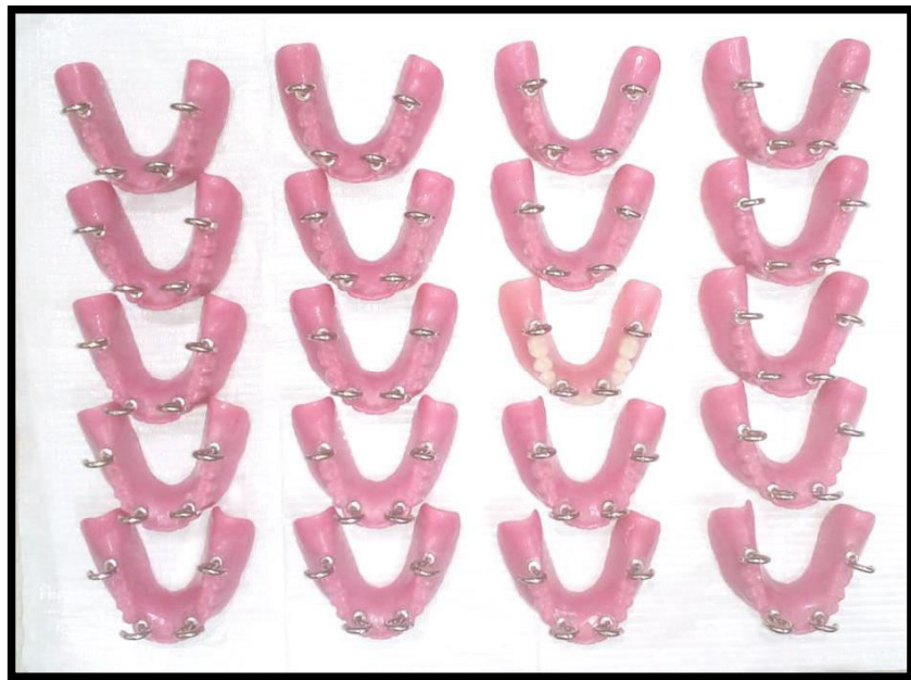
Fig.65 Hooks attached to all the test dentures
