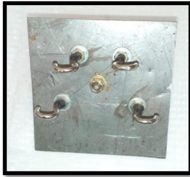
Fig.18 Metal plate with hooks in the bottom side corresponding to the hooks in the denture and one hook in the top side to be attached to the load cell of the universal testing machine
