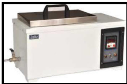
Fig.22 Curing water bath
