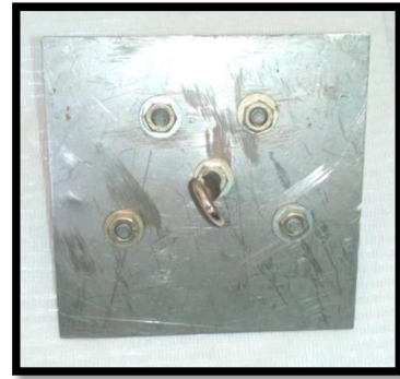
Fig.18 Metal plate with hooks in the bottom side corresponding to the hooks in the denture and one hook in the top side to be attached to the load cell of the universal testing machine
