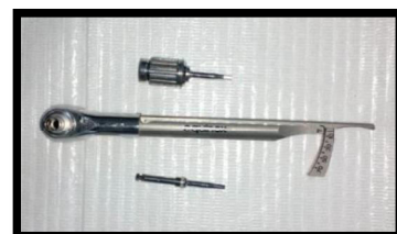
Fig.23 Torque wrench and hex drives
