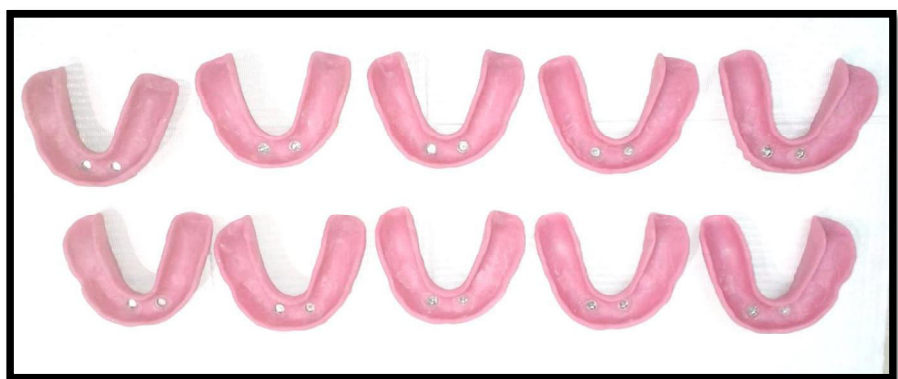
Fig.58 Duplicated test dentures – Intaglio surfaces with metal housings in B and D positions
