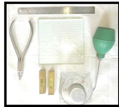
Fig.27 Metal scale, chip blower, glass plate, spirit columns, spirit lamp, universal plier
