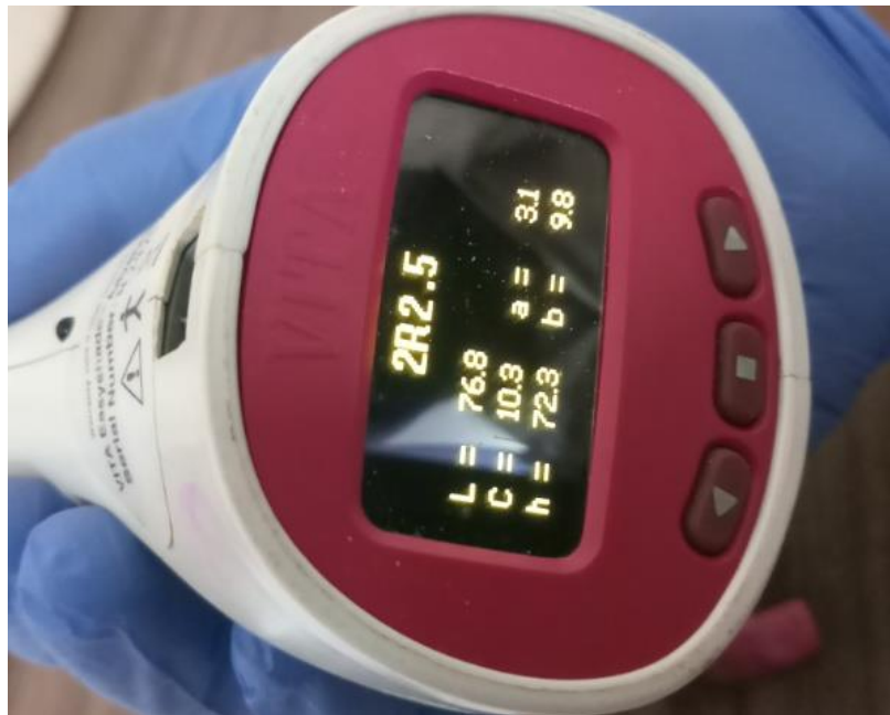
Figure 11: Reading Obtained from spectrophotometer for core specimen
