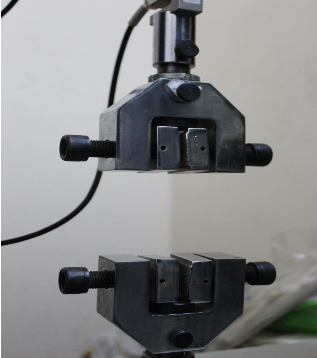
FIGURE NO: 8 UPPER AND LOWER JAW OF UNIVERSAL TESTING MACHINE
