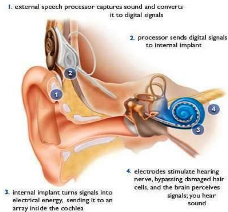
Fig-3.11: Schematic representation of electrical hearing as provided via a cochlear implant
