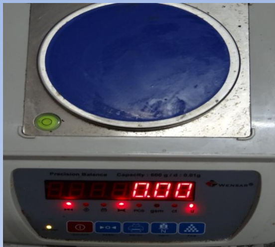
Figure 6a Weighing balance for weighing chemicals for preparing artificial saliva and demineralizing solution
