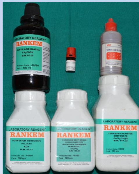
Figure 2b chemicals for preparing demineralizing solution
