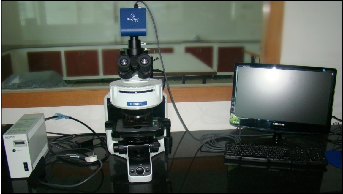
Figure 5- Research Microscope with ProgRes Capture Pro 2.8 Software (Olympus Opto Systems India Pvt. Ltd.)
