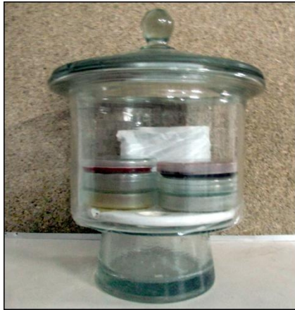
Figure 17- Anaerobic Gas Jar with Poured and Spread Plates
