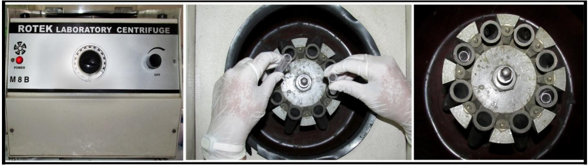
Figure 3- Placement of Test Tube Containing Sample into Centrifuge
