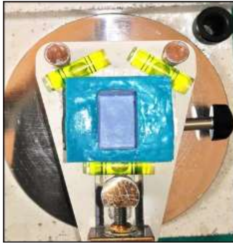
Fig.47: Silicone putty index made parallel to the floor using spirit level indicators
