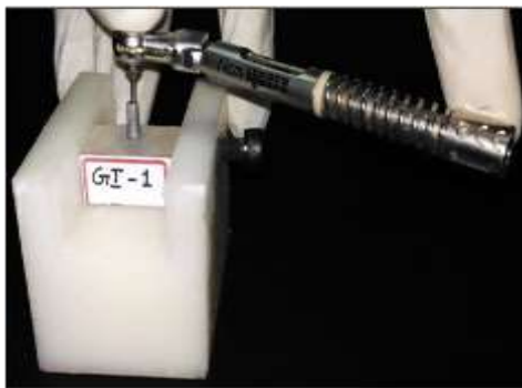
Fig.54a: Retorquing of abutment screw after 24 hours (Group I)
