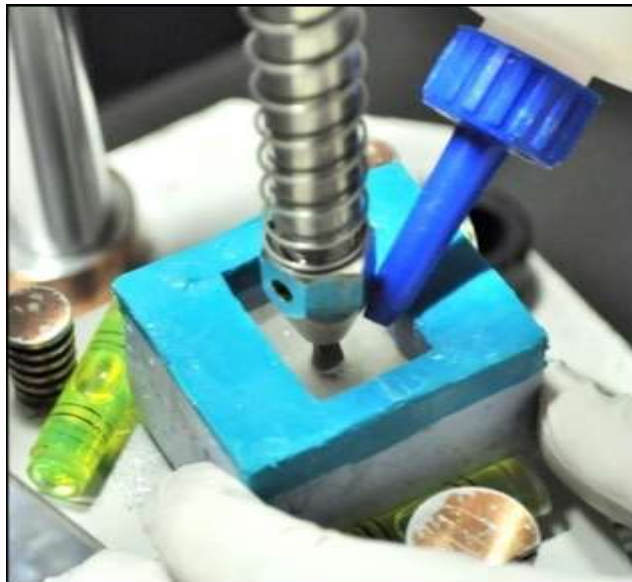
Fig.50a: Pouring of clear acrylic resin into silicone putty index
