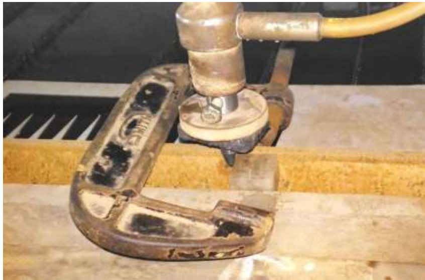
Fig.59: Resin block secured on sectioning platform of water jet sectioning equipment
