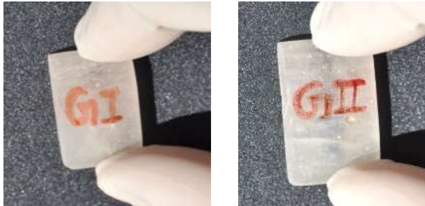
Fig.63a: Cleaning and smoothening of sectioned test sample using silicon carbide emery paper (Group I)
