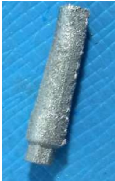
Fig. 42: Laser-sintered abutment after sprue detachment
