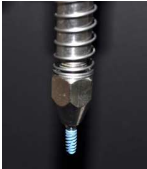
Fig.48: Attaching the connected implant abutment assembly to the mandrel of surveying arm
