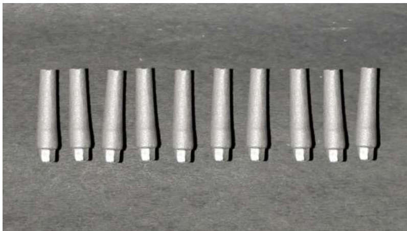
Fig 44: Finished customized laser-sintered Co-Cr abutments
